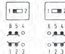
2 changeover contacts switch position
